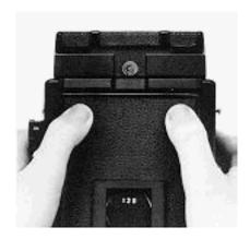
When closing the back cover, firmly press both sides of the back cover, making sure that neither side of the back cover is open or loose. Unless the back cover is closed tightly, the automatic film stopper will not work.
